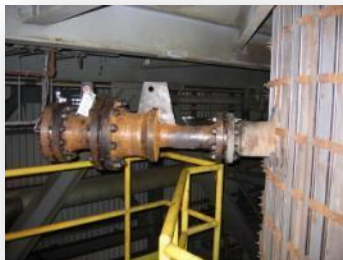
Sapphire fiber temperature sensor testing in TECO coal gasifier
